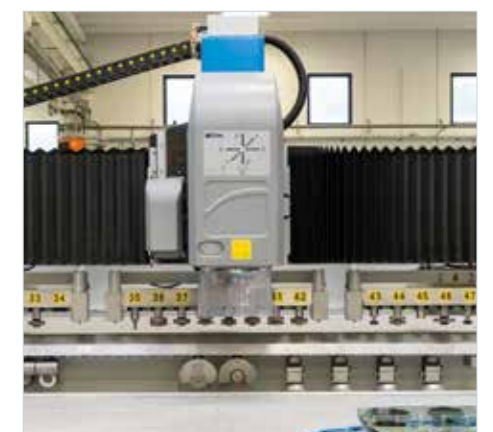
Under-beam tool holder with up to 24 cone positions.
