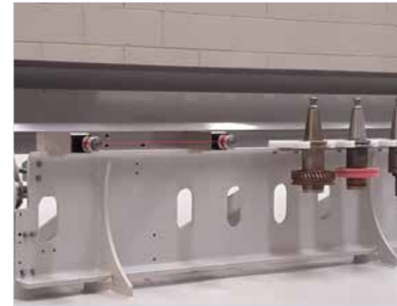
It is possible to install laser presetting in the tool rack for better protection from water and to optimize the use of the table.
